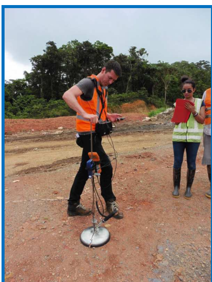
Mr. Richard Gronert from NV AFVALZORG Netherlands using specialised state of art technology to measure methane emissions from the Naboro Landfill.
