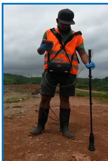
A USP student using specialised instrument to scan the landfill surface for “hotspot” emissions.
